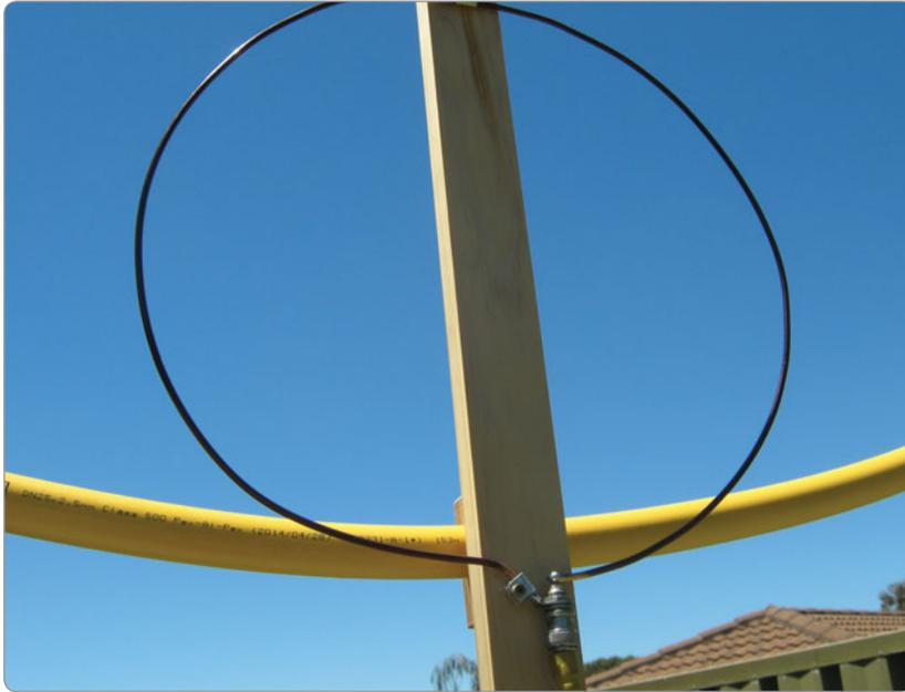
Photo 5: The copper wire driving loop.
