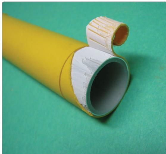
Photo 2: Stripping the end of the plastic pipe.
