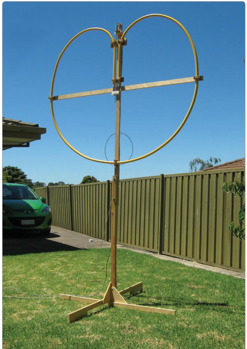
Photo 1: The completed magnetic loop.
