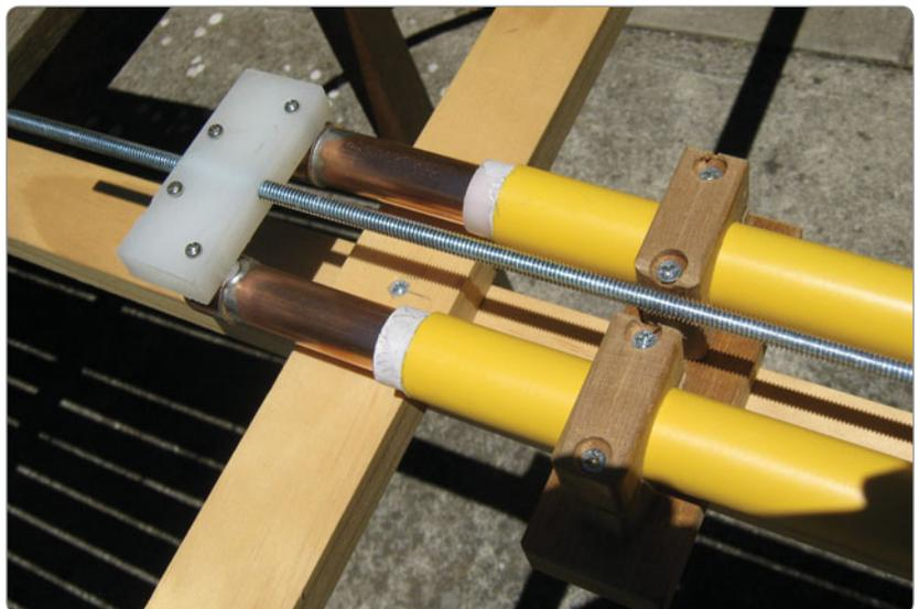
Photo 4: Close up of the timber clamps.
